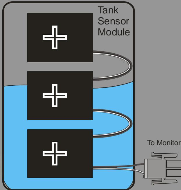
The Tank Sensor features field effect technology, a non-invasive method. Each Sensor array contains three sensors which glue externally to the polymer tank wall with high-grade long life adhesive, at the position and level that the water is to be sensed, thus eliminating the need for calibration. Each Sensor emits an electric field into the tank. When the water level passes by the Sensor, it detects a change in its electric field.
