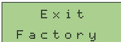
4. Displays Exit Factory option. Press Select to Exit Diagnostics. Press Scroll to continue to return to the first display.
