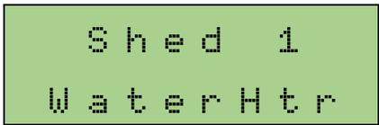
Example: The 1st appliance to be shed is the Electric Water Heater. Most likely it is the least important appliance and will also be the last one to be turned back on. In the case of the Water Heater, the LP heater will heat the water when the Electric Water Heater is shed.
