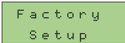
2. Displays Factory Setup option. Press Select to enter Factory Setup review mode. Press Scroll to continue to next menu option.
