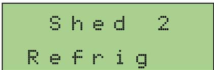
Example: The 2nd appliance to be shed is the Refrigerator. An RV Refrigerator will automatically switch to run off the LP when electric power is removed.
