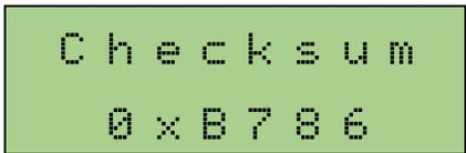
This displays the Checksum of the entire RV Data-2 file. It can be used to confirm any data corruption. RV-Data-2 file contains the personality of the **MIDI-PCS** which includes RV Model specific information like appliances to shed, how they are wired, Generator size, and if 50A service is enabled or disabled.
