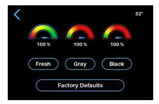
To restore all your tanks to their original factory calibration levels, press the "Factory Defaults" button. The Factory Defaults option can be selected at any time, even if one or more of the tanks are not empty.
